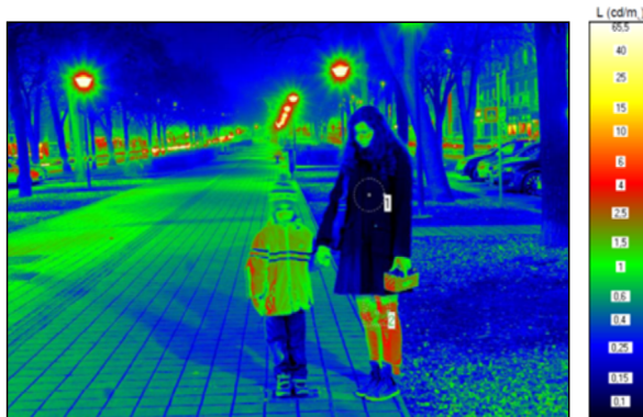
FIGURE 6.4. Measurement of the luminance distribution of the observed environment [6]
