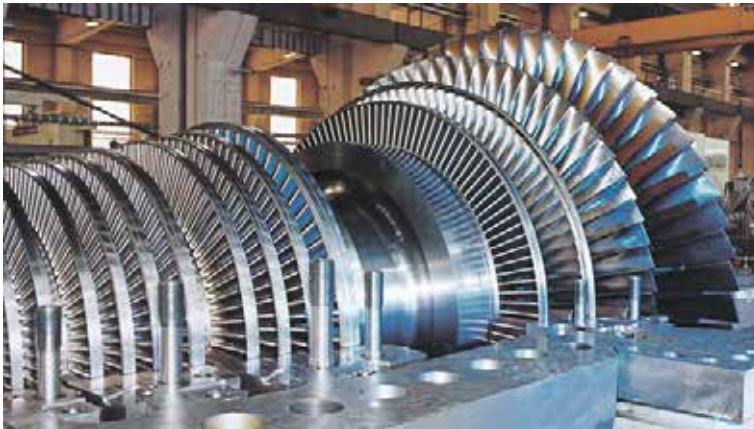
Fig. 7.7. Steam turbine (Source:WEB-4)
