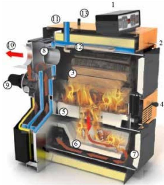
Fig. 6.10. Steel gas generational boiler Caldera Megatherm: 1 – control panel; 2 – start trigger lever; 3 – fuel chamber (furnace); 4 – control levers for primary and secondary air flows; 5 – burner (aerator); 6 – ash collector; 7 – combustion chamber; 8 – shut-off valve; 9 – smoke extraction fan; 10 – flame – gas flow direction of furnace; 11 – water supply to the system; 12 – cooling coil; 13 – connecting the cooling coil (Source: WEB-3)
