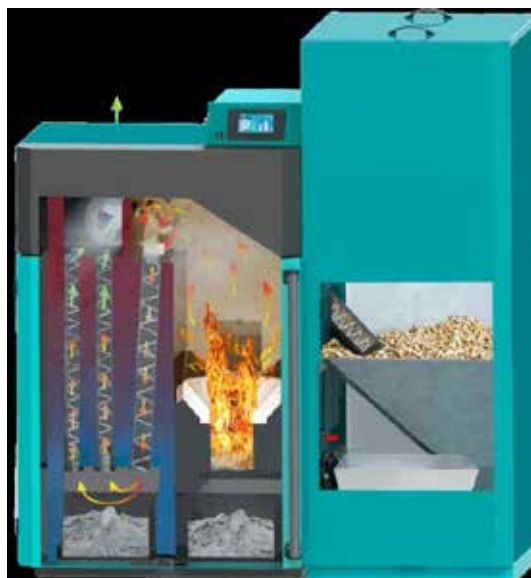
Fig. 6.13. Pellet boiler (Source: WEB-6)
