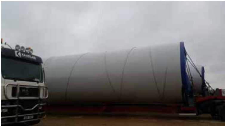
Fig. 3.12. Transportation and storage of wind turbine towers during the building of a wind turbine (farm) (Source: photos by T. J. Teleszewski (A) and K. Jasiūnas (B))
