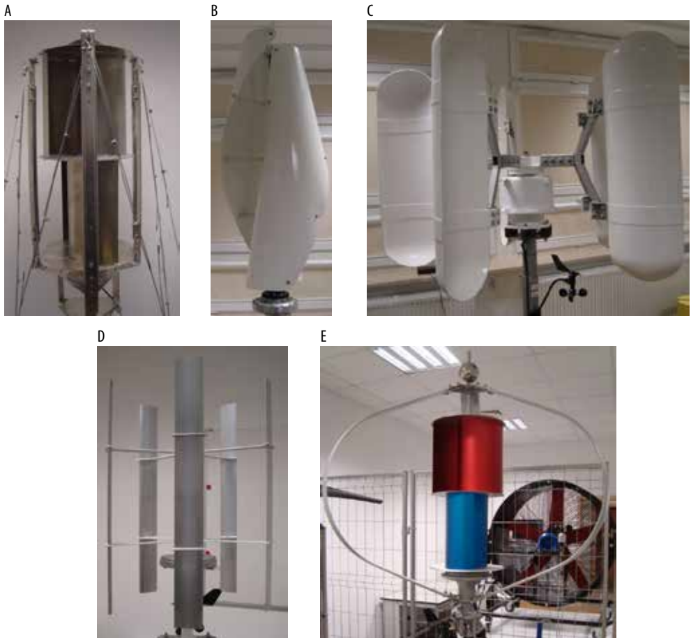
Fig. 3.23. Types of vertical axis wind rotors: A) Savonius rotor, B) Spiral rotor, C) C-rotor type, D) rotor Darrieus H, E) combined Savonius and Darrieus rotors (Source: photos by T.J. Teleszewski)
