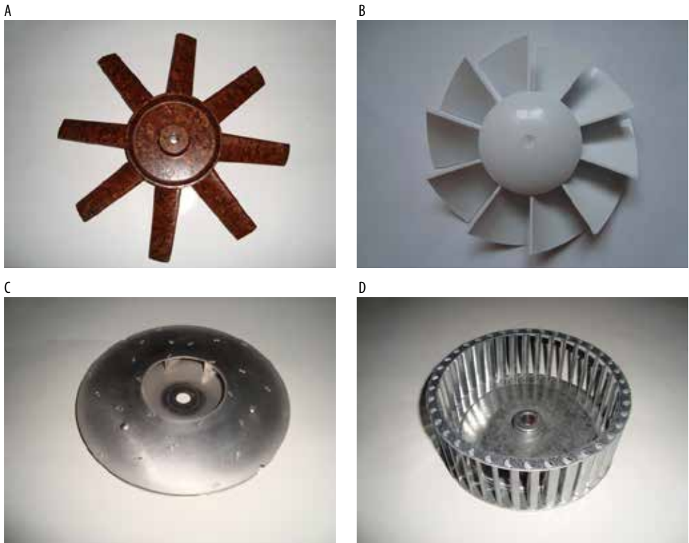
Fig. 8.8. Examples of fan rotor designs: A), B) axial fan impellers, C) a centrifugal impeller, D) a cross flow fan impeller (Source: photos by T.J. Teleszewski)
