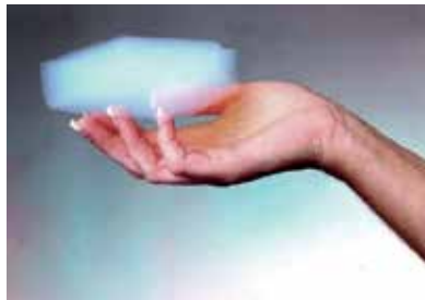
Fig. 3.14. Pure aerogel sample (Source: WEB-6)
