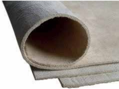
Fig. 3.15. Continuous filament glass fibre (Source: WEB-5)
