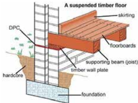
Fig. 3.6. A suspended timber floor (Source: WEB-2)
