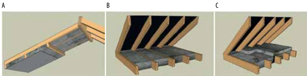
Fig. 3.7. Laying thermal insulation in buildings with an attic: A) in the roof slope and additionally under the rafters, B) between ceiling joists, C) between and over ceiling joists (Source: WEB-3)
