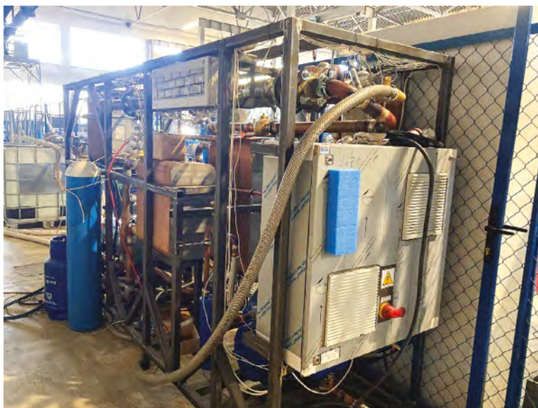
FIGURE 7. Photo of the tested hybrid refrigeration unit
