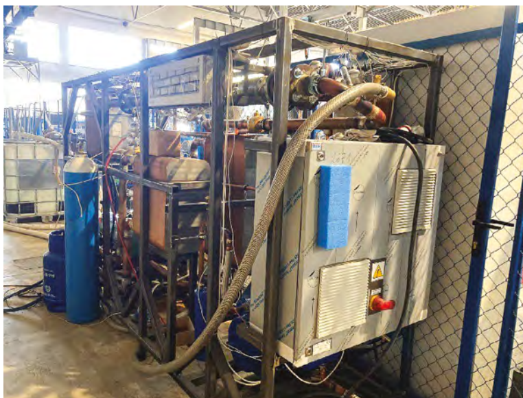
FIGURE 7. Photo of the tested hybrid refrigeration unit
