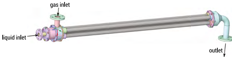
FIGURE 2. The CAD model of the tested jet-ejector scrubber for 40 kW engine
