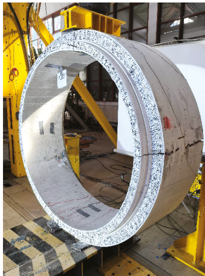
FIG. 1. Prefabricated concrete ring prepared for crushing testing with the application of an optical displacement measurement system
