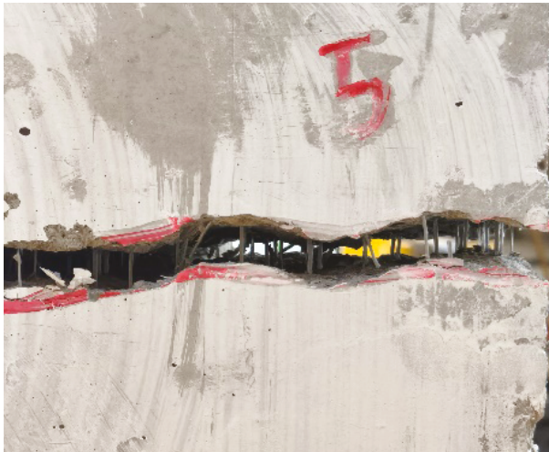
FIG.2. Failure crack in a fibre-reinforced concrete ring after the crushing test
