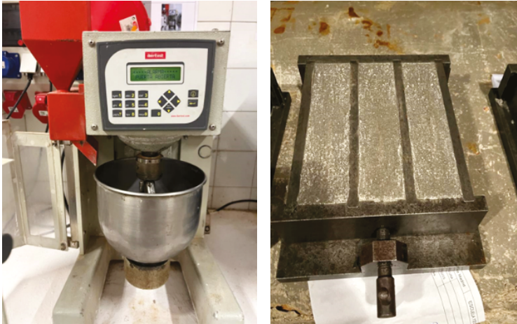
FIG. 1. Sustainable mortar mixing process. Standardized mold (40x40x160 cm) placed in a humid chamber
