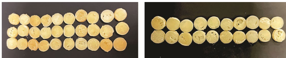
Figure 5. 3D printed samples with 100% and 75% infill
