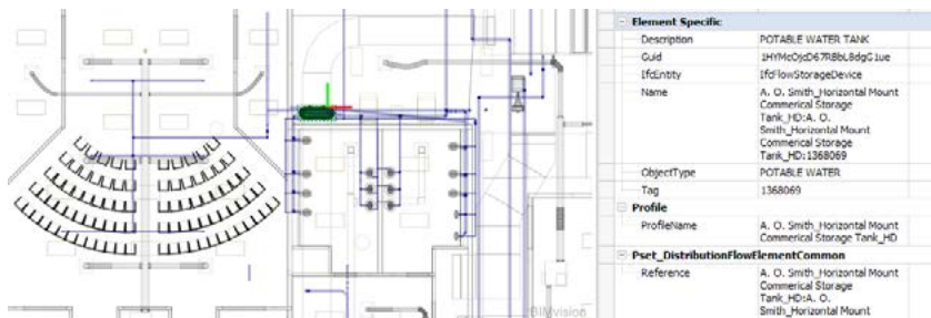
Figure 2: Location of the water tank on the floor, with additional information included in the BIM model. The model viewed in the BIMvision viewer. Prepared using the OTC Conference Center building model provided by Autodesk Inc. (Autodesk, 2022).
