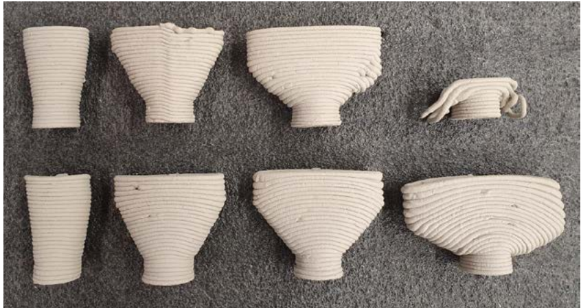
Figure 8: Top row displays planarly printed objects and bottom one non-planarly sliced ones. Overhangs of 10, 30, 50 and 70 degrees are shown.
