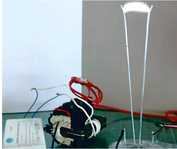
FIG. 6.6. Jacob's Ladder – rising arc ( www.youtube.com/watch?v=6hhaaSSCU5k )
