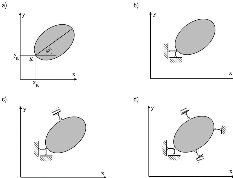
Fig. 1.1. The planar body and the constraints.
