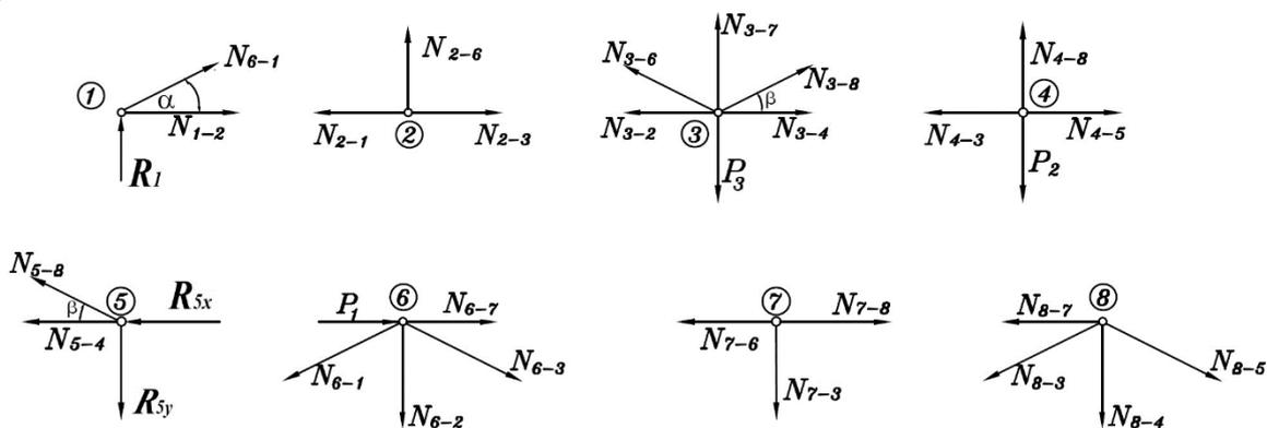
Fig. 2.6.6. Planar truss – method of joints.
