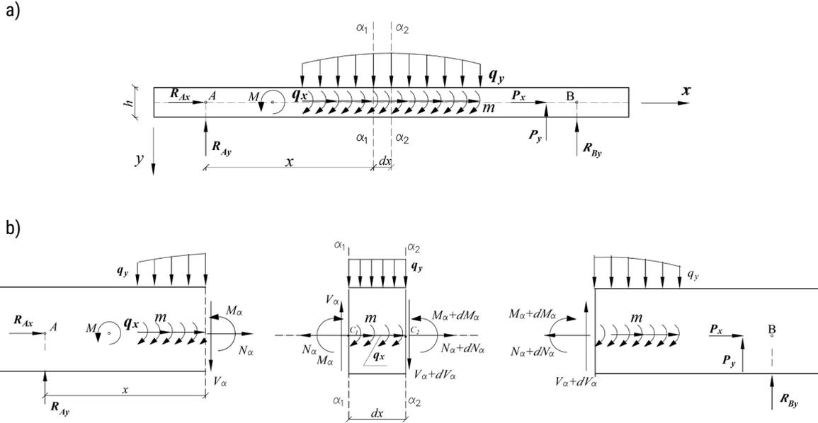
Fig. 2.2.1.1. a) Beam with arbitrary distributed loading, b) Differential beam element [4].
