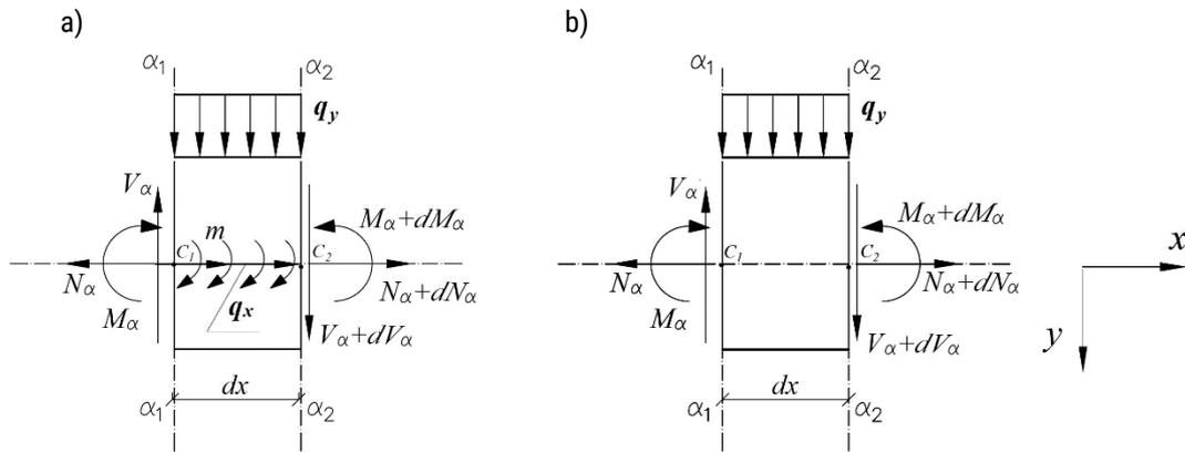
Fig. 2.2.1.2. Differential beam element.
