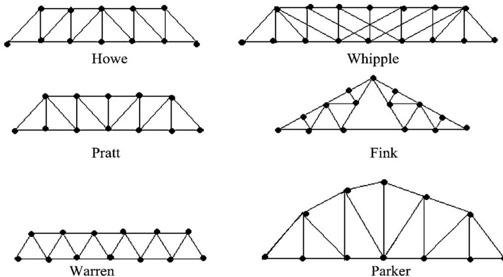
Fig. 2.6.1. Examples of named truss [1].
