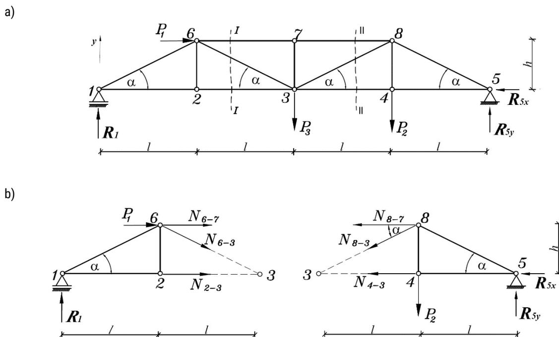
Fig. 2.6.7. Planar truss – method of sections.
