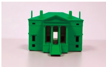
FIG. 2.12. Models were made with a 3D printer MARKETBOT REPLICATOR TM 2 DESKTOP 3D PRINTER PALLADIO HOUSES VILLA CHIERICATI (Source: own elaboration, 2020)
