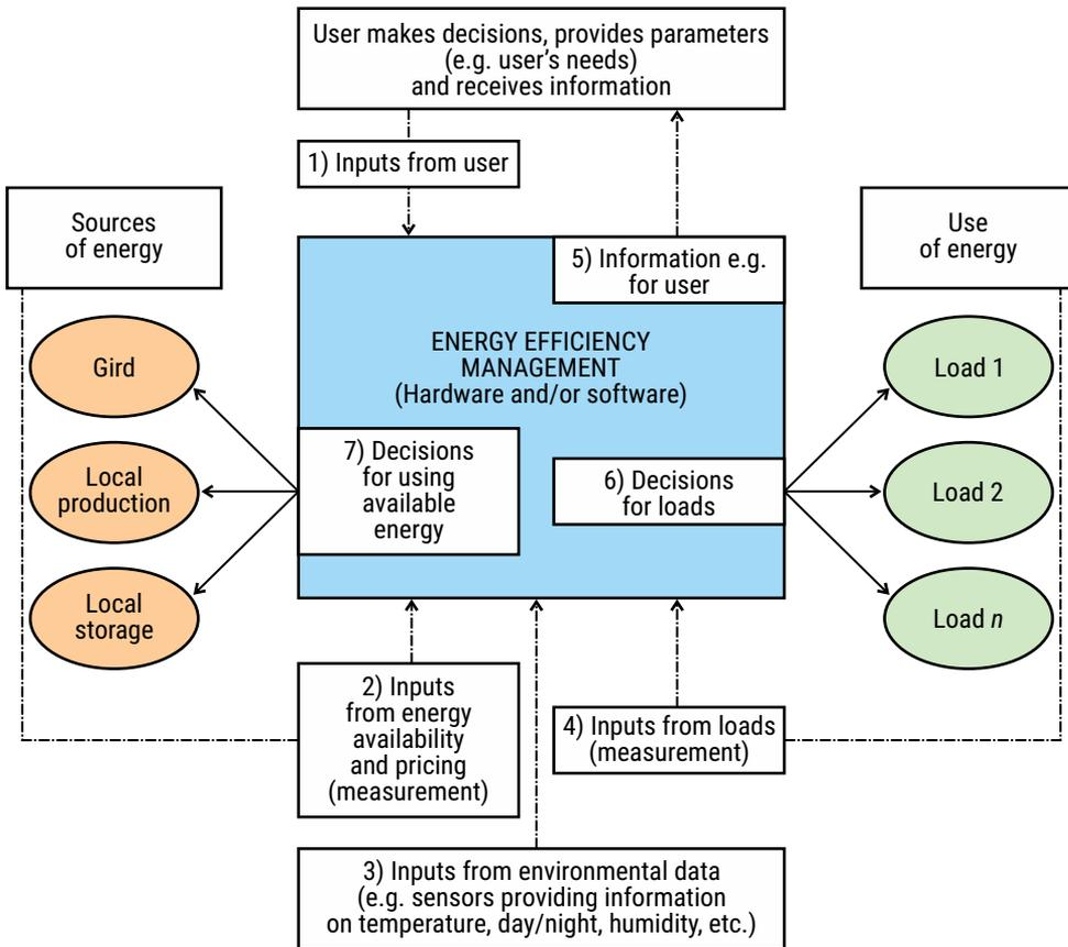
FIGURE 7.3. Energy efficiency and load management system overview.
