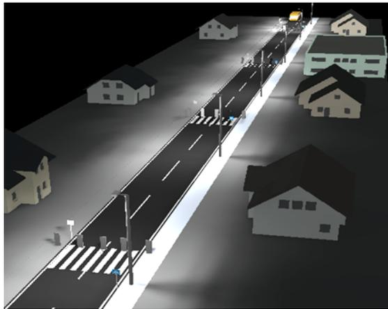
FIGURE 6.5. View of the road lighting project in the DIALux software
