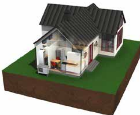
Fig. 5.28. An example of the air heat pump in a building (Source: Smuczyńska, 2015)
