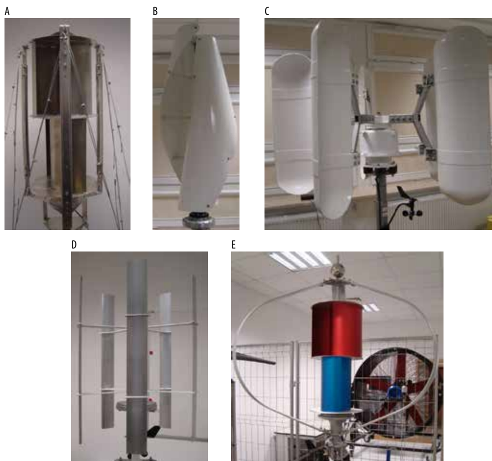
Fig. 3.23. Types of vertical axis wind rotors: A) Savonius rotor, B) Spiral rotor, C) C-rotor type, D) rotor Darrieus H, E) combined Savonius and Darrieus rotors (Source: photos by T.J. Teleszewski)
